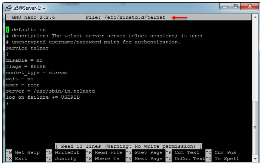
The screenshot shows a terminal window titled "u5@Server-1: ~". The window displays the contents of the file "/etc/xinetd.d/telnet". The file contains the configuration for the telnet service, including default settings, a description, and the path to the server executable. The terminal window has a red arrow pointing to the file name in the title bar.
